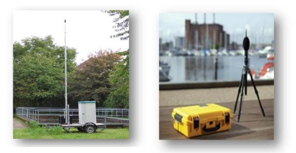
Figure 18: Noise Monitoring Terminals (NMTs) – on trailer (left), portable (right)
