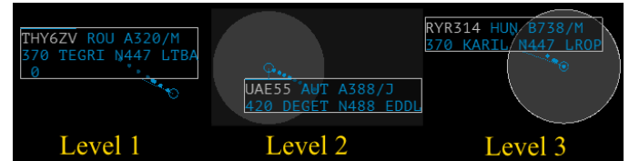
Figure 1. Screenshots of the three escalation levels' visual cues for a handover event.
