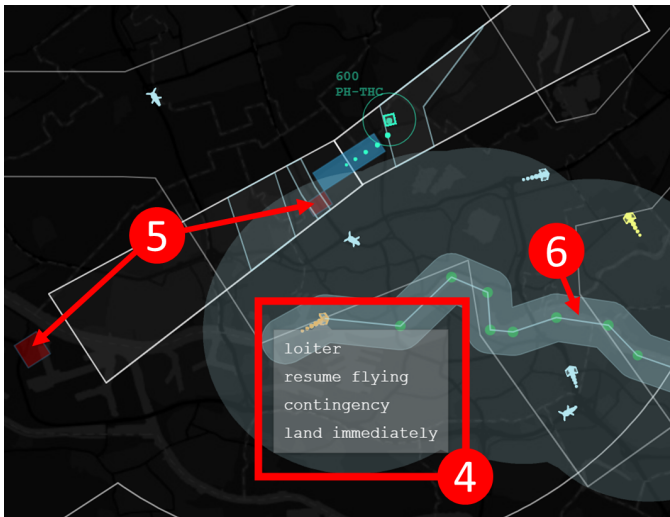
Figure 2. Overview of new UAS intervention tools incorporated into the collaborative ATM-UTM interface for tower controllers.
