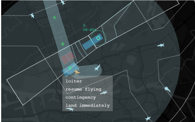
(b) Use of UAS-specific commands to manage conflicts in the active control strategy.
