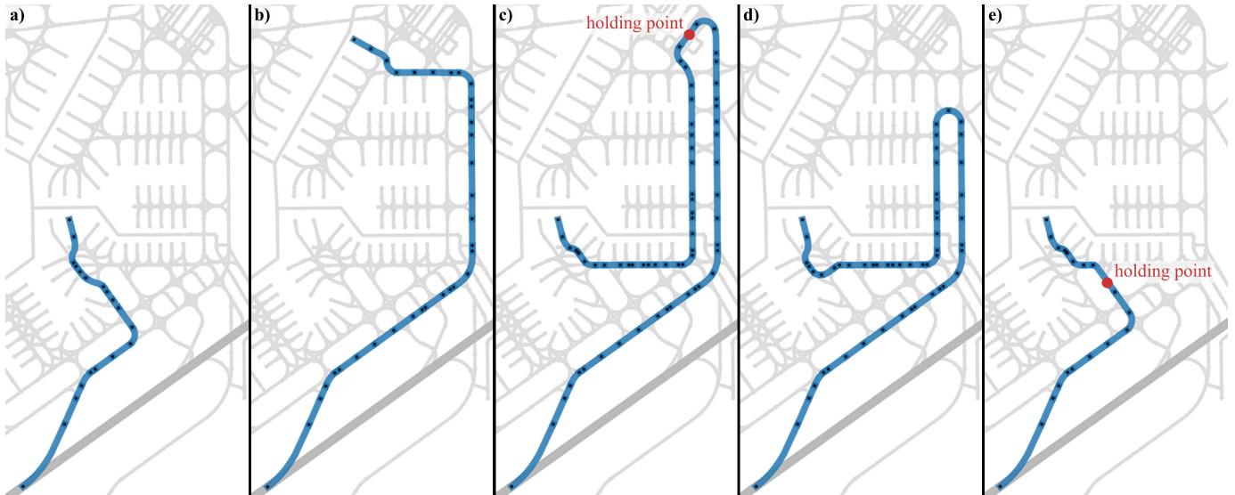
Figure 8. The stand of an arriving aircraft is unavailable: SAMP paths of a) original route, b) rerouting to a different stand, c) holding at a remote holding point, d) detour with minimal speed, and e) holding at a non-standard holding point
