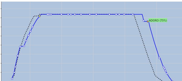
Figure 7. Agreed trajectory with a constraint probability vs flown trajectory.
