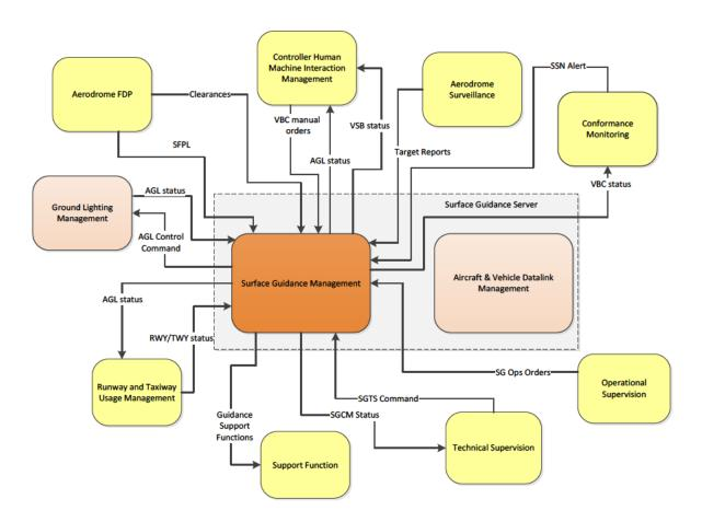
Figure 5: SGS Interactions - View of Surface Guidance Management
