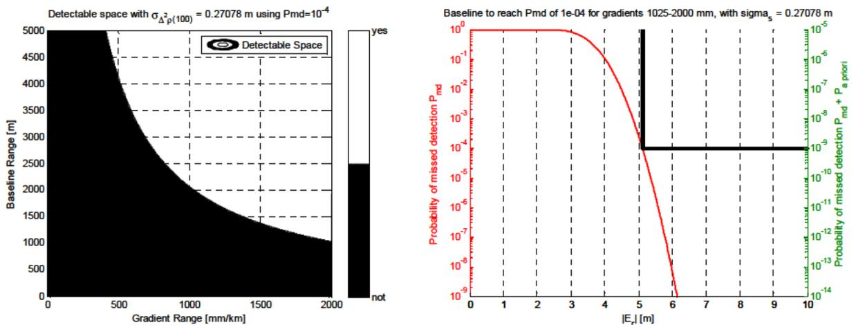
**Figure 5-22: Detectable space for a code based absolute gradient monitor for  $P_{md} = 10^{-4}$  (left) and resulting  $P_{md}$  for code based absolute ionospheric gradient methods assuming a detection need for gradients larger 1000 mm/km (right)**
