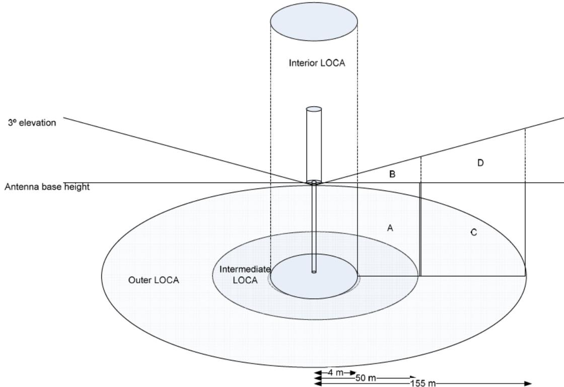
**Figure 4-2 LOCA for the combination of multipath limiting antenna and 0.1 chip E-L narrow correlator**
