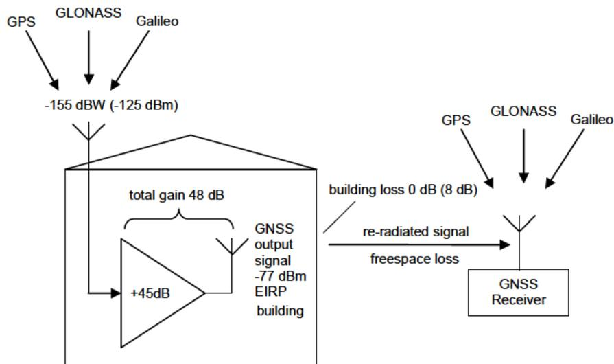
Figure 5-3: Proposed European technical standard for GNSS repeaters
