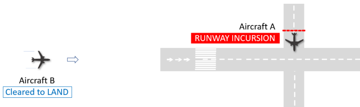
Figure 12: CMAC RUNWAY INCURSION Alert caused by Aircraft A entering RPA without clearance and Aircraft B given LAND by ATCO triggers a CMAC vs Clearance Alert .
