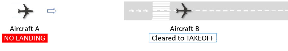
Figure 14: CMAC NO LANDING Clearance Alert caused by Aircraft A landing without clearance and Aircraft B given TAKEOFF by ATCO triggers a CMAC vs Clearance Alert .
