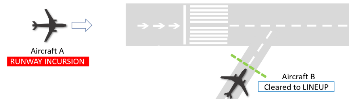
Figure 11: RMCA caused by Aircraft A landing soon without LAND clearance and Aircraft B given LINE UP by ATCO triggers a RMCA vs Clearance Alert
