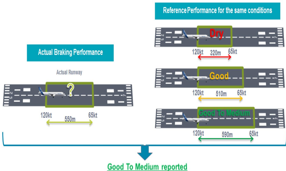
Figure 2: Technology used for identifying the runway condition encountered during landing
