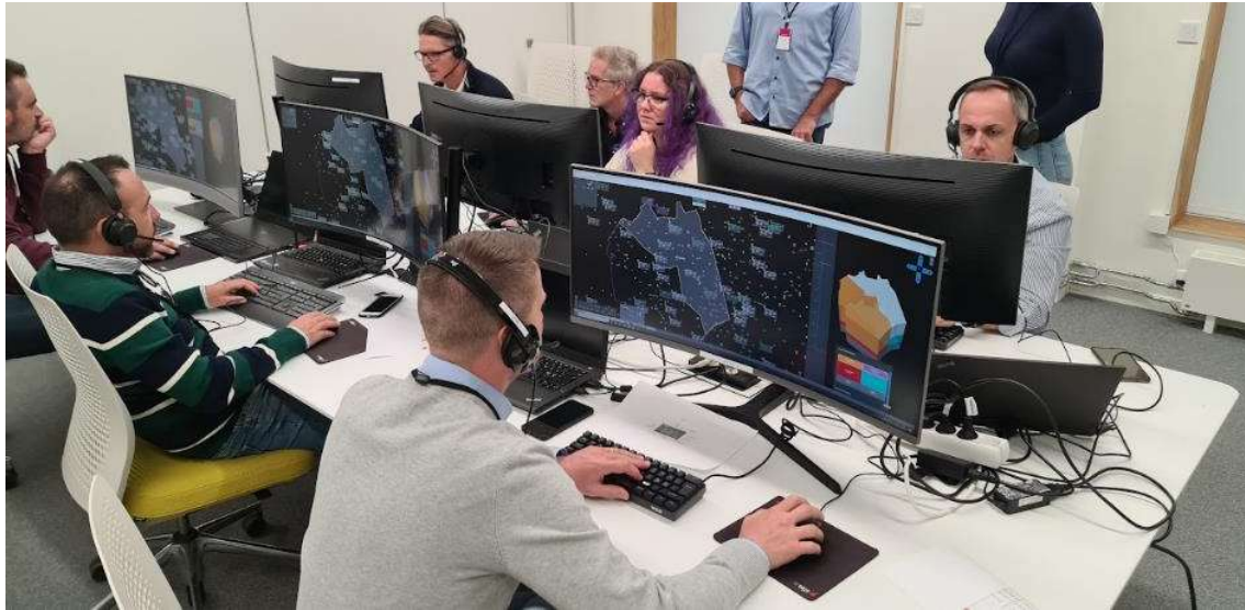
Figure 74 – Set-up of SIMADES CWP for five ATCO positions and a master controller
