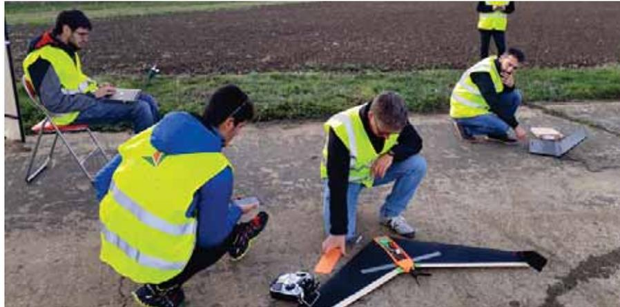
Reducing the risk of conflict between airspace users becomes more important as more drones enter the airspace. The Clear Air Situation for uaS (CLASS) project examined the potential of ground-based technologies to detect and monitor cooperative and non-cooperative drone traffic in real-time. The consortium fused surveillance data obtained using a drone identifier and tracker, and holographic radar, to feed a real-time UTM display.
