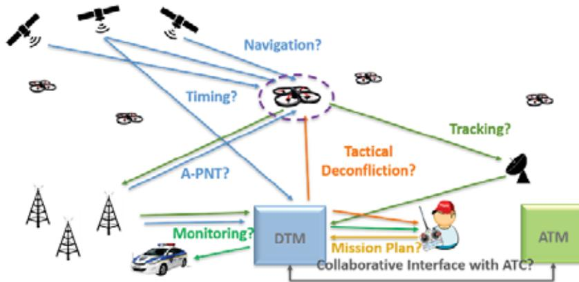
The current communications, navigation and surveillance (CNS) infrastructure is designed to support the needs of manned aviation. The requirements of the emerging drone sector are different and will rely on new and existing technologies to perform effectively. The TERRA project set out to identify relevant ground technologies and to propose a technical ground architecture to support drone operations.
