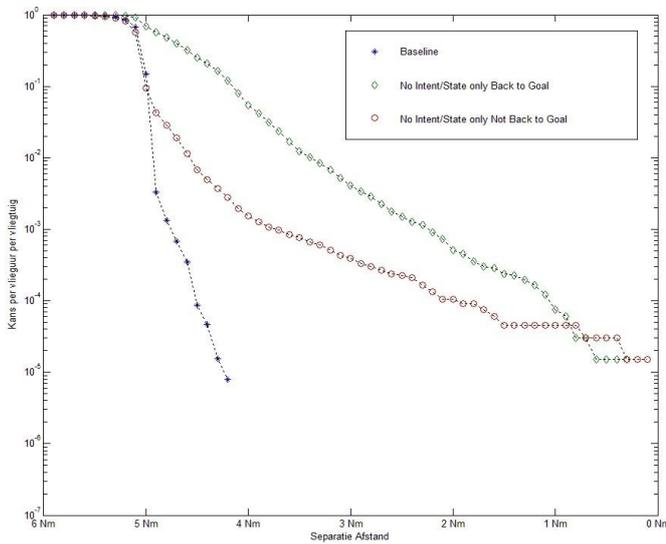
Figure 8. What happens when the MTCR layer is left out, by which the STCR layer has to do all conflict resolution. The curves show baseline results (+), STCR only (o) and STCR extended with a back to goal algorithm (diamonds).
