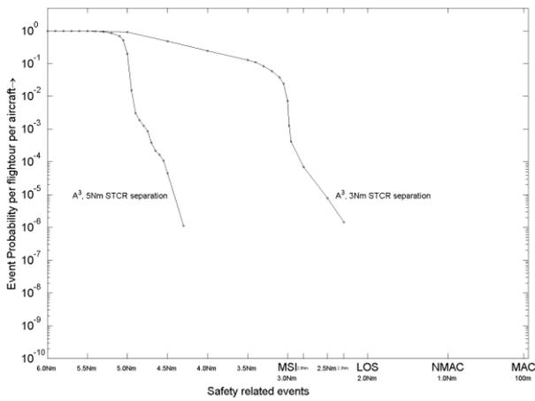
Figure 2. Estimated event probability per aircraft per flight hour for random traffic under  $A^3$  model control at 3x high 2005 en-route traffic demand. Left curve shows effect of 5 Nm STCR separation.
