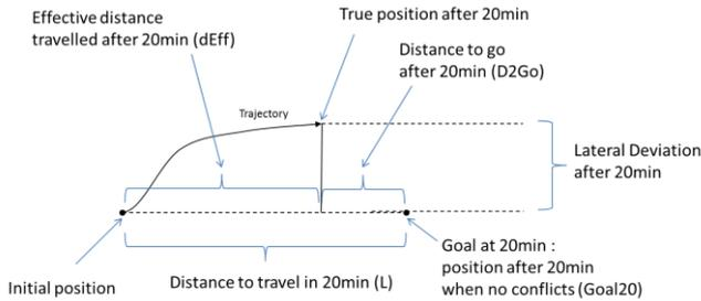
Figure 5. Flight efficiency measures.
