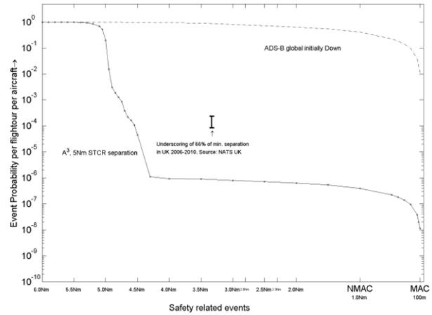
Figure 3. Estimated event probability per aircraft per flight hour for random traffic under  $A^3$  model control at traffic demand of 3x high en-route traffic demand in 2005. The dashed curve at the top is obtained through running standard MC simulations for the  $A^3$  ConOps model under the initial condition that ADS-B Global is Down. This curve has been used to construct a completion of the line curve for miss distance values below 4Nm.
