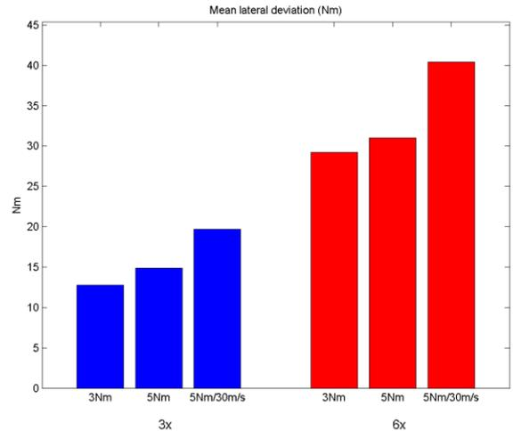
Figure 7. Mean absolute value of lateral deviation for airborne absolute self separation TBO concept under 3x and 6x high 2005 traffic demands.
