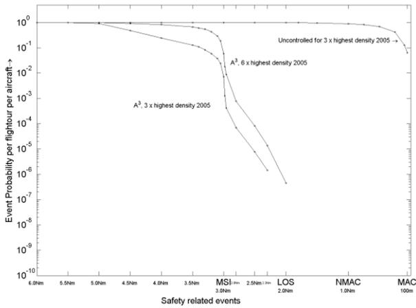
Figure 1. Estimated event probability per aircraft per flight hour for random traffic under  $A^3$  model control and uncontrolled. Traffic densities are 3x and 6x high en-route traffic density in 2005.
